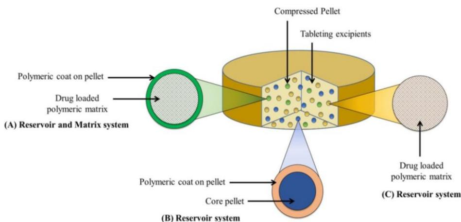
**Fig. 4:** MUPS constructed from pellets made from the reservoir, matrix, and combined pellet system<sup>19</sup>
