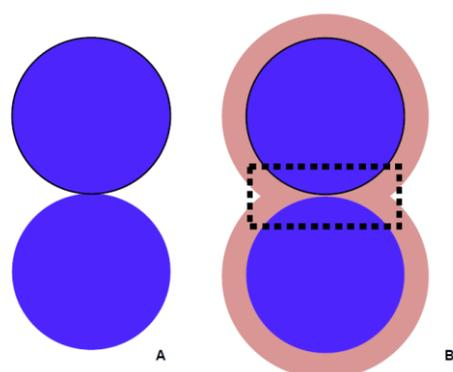
**Fig. 3:** Profile of tablet bond without coating system (A) and with coating system (B)<sup>22</sup>
