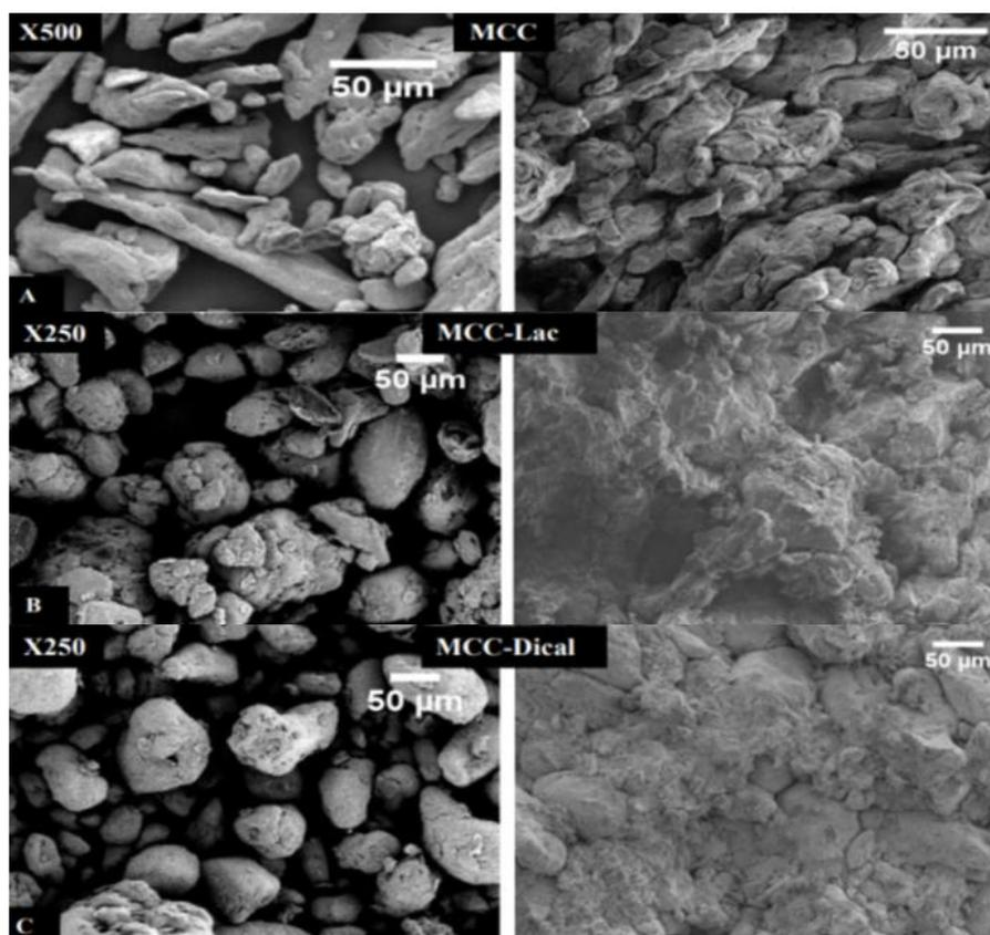
**Fig. 9:** Scanning Electron Microscope (SEM) before compression (left panel) and after compression (right panel) from (A) MCC (B) MCC-lactose (C) MCC-Dical granules<sup>35</sup>.
