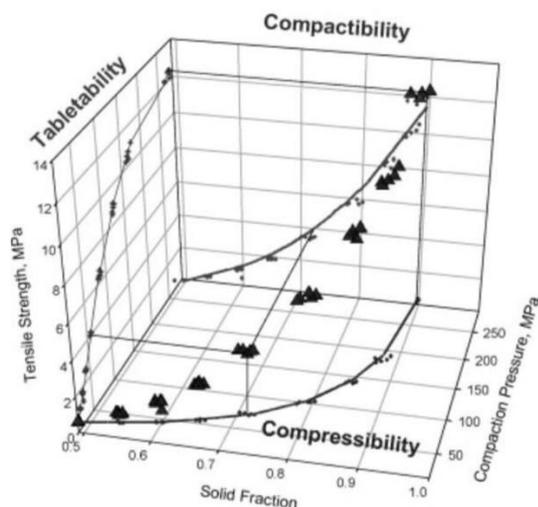
**Fig. 1:** The correlation between compactibility, compressibility, and tableability in a scheme<sup>13</sup>.
