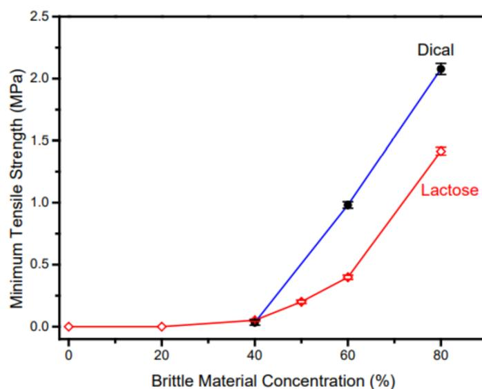
**Fig. 8:** The effect of MCC binder combined with lactose and Dical excipients on tensile strength<sup>35</sup>
