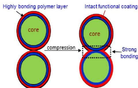
**Fig. 5:** The contact area between particles after coating and compression<sup>35</sup>
