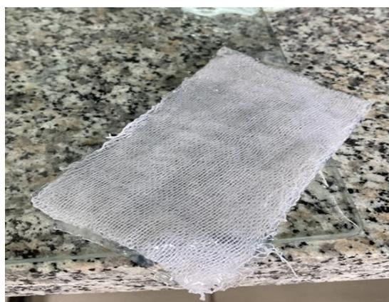
**Fig. 2:** Sodium alginate film loaded with Zinc nanoparticles.
