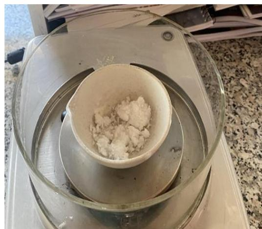
**Fig. 1:** yield of zinc oxide nanoparticles.
