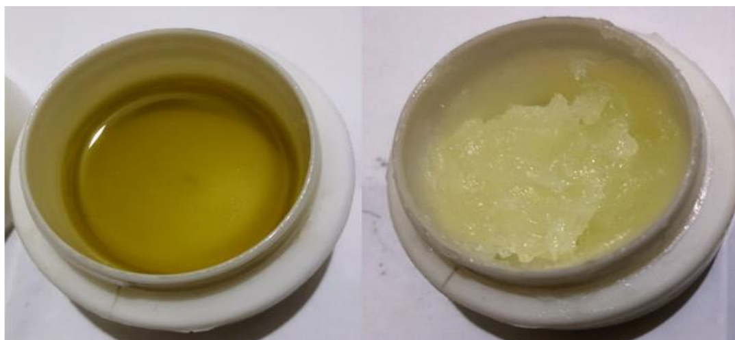
Fig. 4: Olive oil before (on the left) and after ozonation (on the right) with the change in its density and viscosity.
