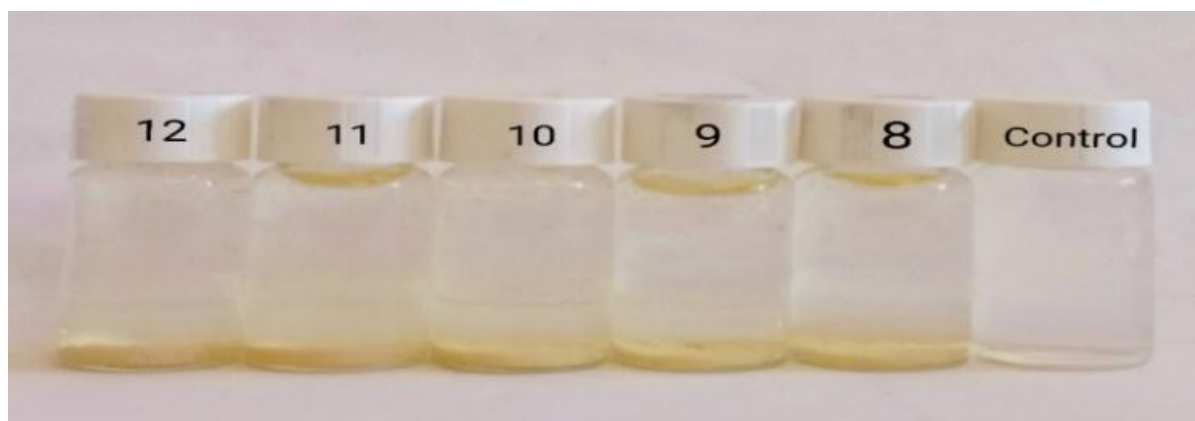
Fig. 13: Digital photograph showing the effect of 5 tested pH values (8, 9, 10, 11, and 12) on the biosynthesis of ZnO NPs compared to a negative control.
