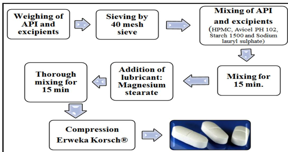
**Fig. 2:** Diagrammatic representation of the direct compression tablet manufacturing process.
