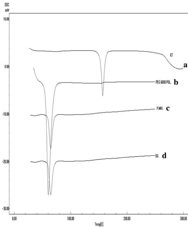
**Fig. 18:** Shows DSC thermograms of (a) pure drug KT, (b) PEG 6000 polymer, (c) physical mixture of KT with PEG 6000 1:7, (d) solid dispersion of KT with PEG 6000 1:7.
