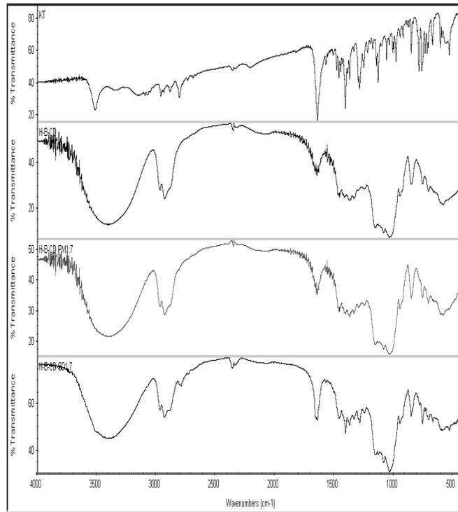
**Fig. 10:** Comparative study of the FTIR spectra of (a) pure drug KT; (b) HP- $\beta$ -CD polymer; (c) P.MIX. 1:7; and (d) SD. 1:7.
