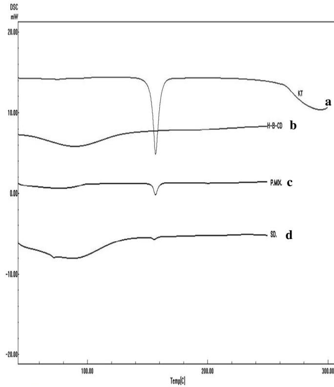
**Fig. 15:** Shows DSC thermograms of (a) pure drug KT, (b) HP-β-CD polymer, (c) physical mixture of KT with HP-β-CD 1:7, (d) solid dispersion of KT with HP-β-CD 1:7.
