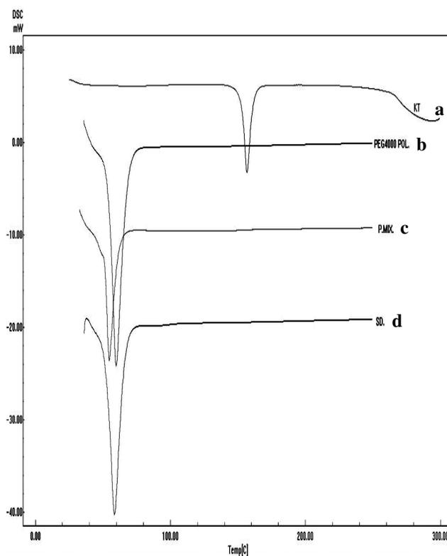
**Fig. 19:** Shows DSC thermograms of (a) pure drug KT, (b) PEG 4000 polymer, (c) physical mixture of KT with PEG 4000 1:7, (d) solid dispersion of KT with PEG 4000 1:7.
