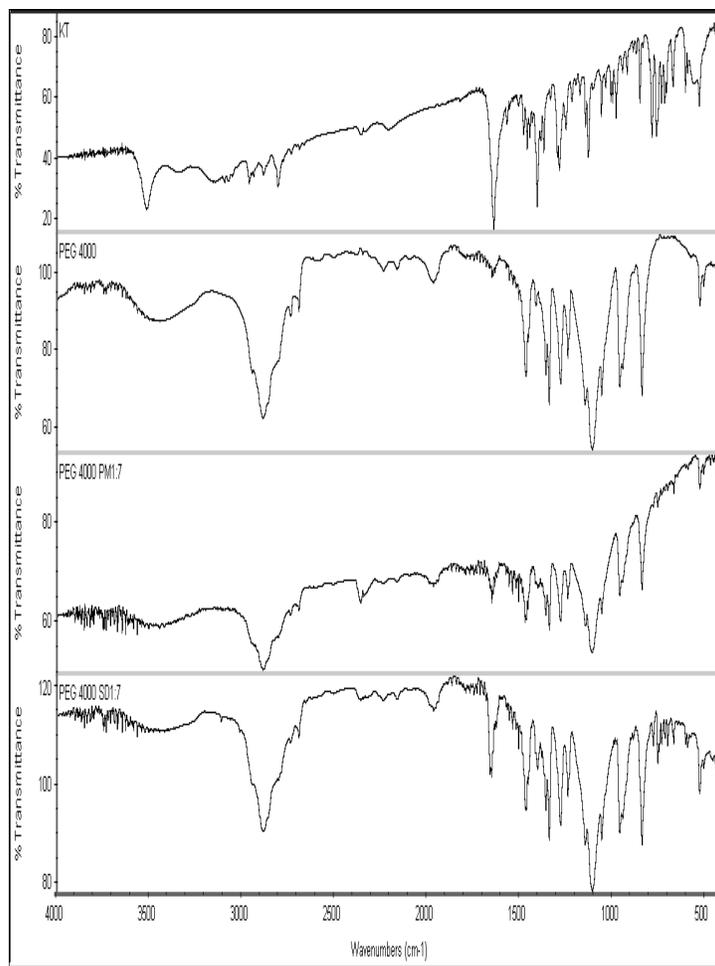
**Fig. 14:** Comparative study of the FTIR spectra of (a) pure drug KT; (b) PEG 4000 polymer; (c) P.MIX. 1:7; and (d) SD. 1:7.
