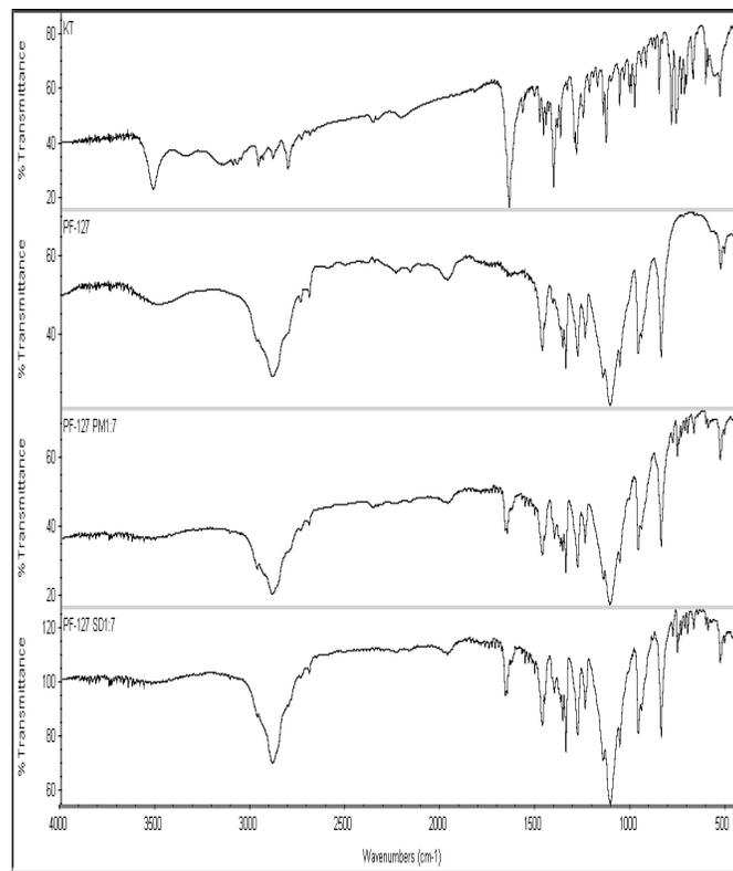
**Fig. 11:** Comparative study of the FTIR spectra of (a) pure drug KT; (b) PF-127 polymer; (c) P.MIX. 1:7; and (d) SD. 1:7.
