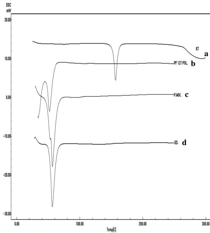
**Fig. 16:** Shows DSC thermograms of (a) pure drug KT, (b) PF-127 polymer, (c) physical mixture of KT with PF-127 1:7, (d) solid dispersion of KT with PF-127 1:7.
