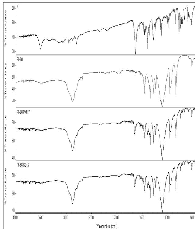
**Fig. 12:** Comparative study of the FTIR spectra of (a) Pure drug KT; (b) PF-68 polymer; (c) P.MIX. 1:7; and (d) SD. 1:7.
