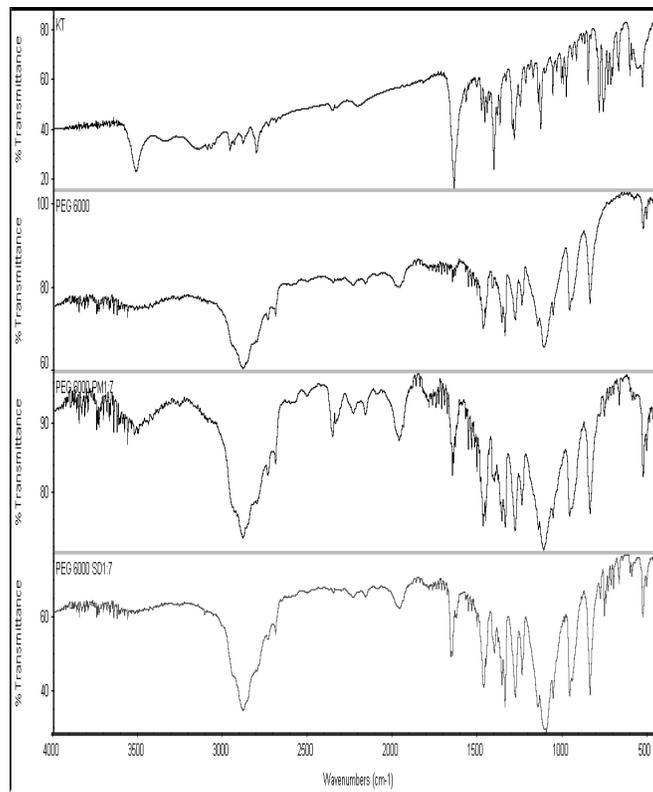
**Fig. 13:** Comparative study of the FTIR spectra of (a) pure drug KT; (b) PEG 6000 polymer; (c) P.MIX. 1:7; and (d) SD. 1:7.
