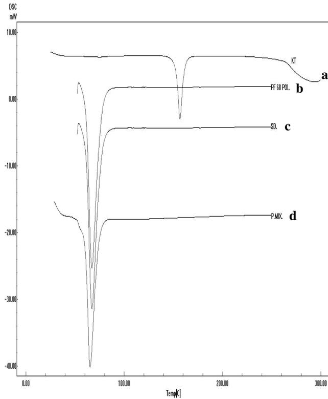
**Fig. 17:** Shows DSC thermograms of (a) pure drug KT, (b) PF-68 polymer, (c) solid dispersion of KT with PF-68 1:7, (d) physical mixture of KT with PF-68 1:7.
