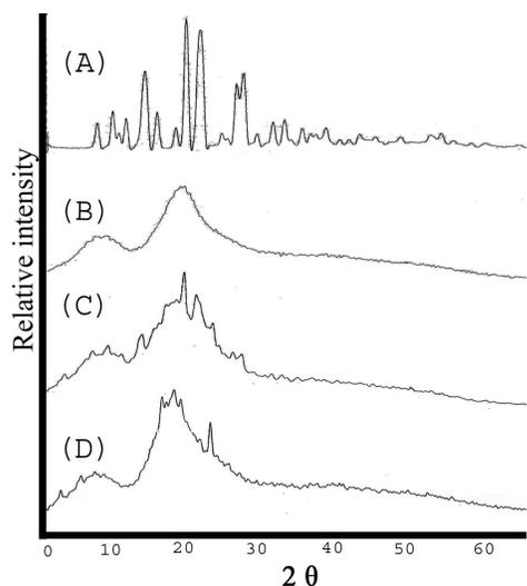
**Fig. 20:** Powder X-ray diffractograms of (A) pure drug KT, (B) HP- $\beta$ -CD polymer, (C) physical mixture of KT with HP- $\beta$ -CD 1:7, and (D) solid dispersion of KT with HP- $\beta$ -CD 1:7.
