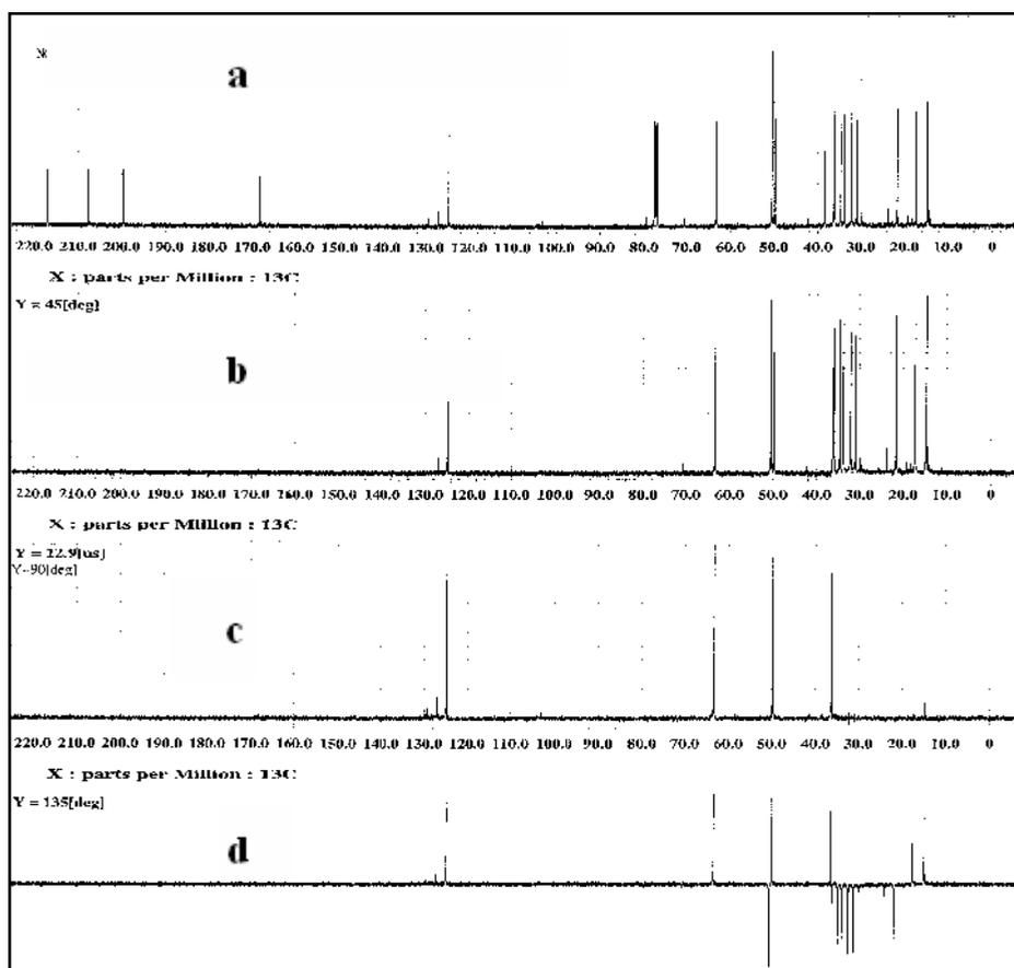
**Fig. 1:**  $^{13}\text{C}$ -NMR spectrum (a) DEPT spectra at  $45^\circ$  (b),  $90^\circ$  (c) and at  $135^\circ$  (d) of  $\mathbf{m}_1$ .
