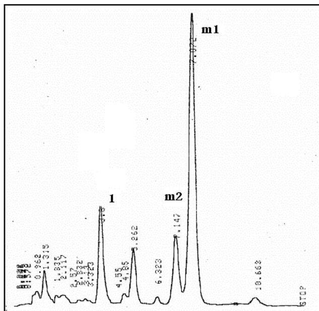
**Fig. 4:** HPLC chromatogram of the reaction mixture illustrating the relative concentration of **1** and its metabolites **m<sub>1</sub>** and **m<sub>2</sub>** after 48 h.
