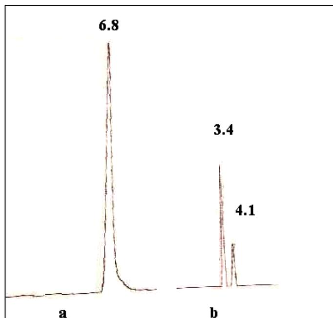
**Fig. 3:** Analytical HPLC profiles of metabolites  $m_2$ : (a) Rp C-18 column,  $\text{CH}_3\text{CN}:\text{H}_2\text{O}$  (2:3); (b) chiral column isopropanol: *n*-hexane (1:50).
