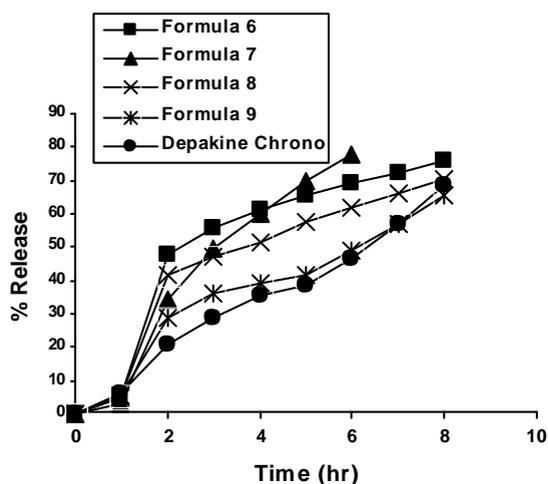
**Fig. 2:** Effect of different binders on the release profile of SV from Valdisoval coated tablets in 0.1 N HCl for 1 hour followed by phosphate buffer, pH 6.8.
